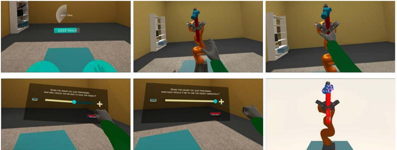
Fig. 4. Sample trial in our experiment. Top row, left to right: The participant waits with their hands in the designated spheres. Then they reach for the object presented by the robot and grasp it; the detected contact points are highlighted in cyan but were not visible during the study. Bottom row, left to right: The user answers Q1 and Q2 about the grasp they just performed. The final picture shows an aggregate of the contact points of multiple users for this scene.
